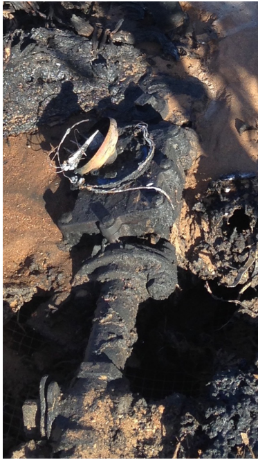
A burnt 2-inch meter (left) and fire hydrant (right) from 2017 Lilac Fire show wildfire's adverse effects on water infrastructure.
